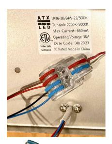
Connect the 4 wires from the Signature Fixture to 2 wires for the AL-WS-DR1 this results In 3500K temperature
